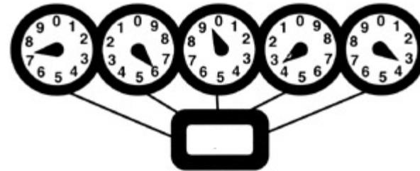
When a pointer rests directly on a number, as in the fourth dial from the right of this example, be sure to check the next dial to the right. If that pointer has not passed zero, as shown here, the number on the previous dial has not yet been reached. Therefore, the fourth dial from the right above should be read as five, not six.
