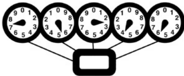
When the needle is between two numbers, always read the smaller of the two numbers. On the right hand dial, read the number that the pointer has just passed and write the number here 5.
